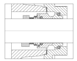
Uncooled stuffing box without internal barrier fluid
