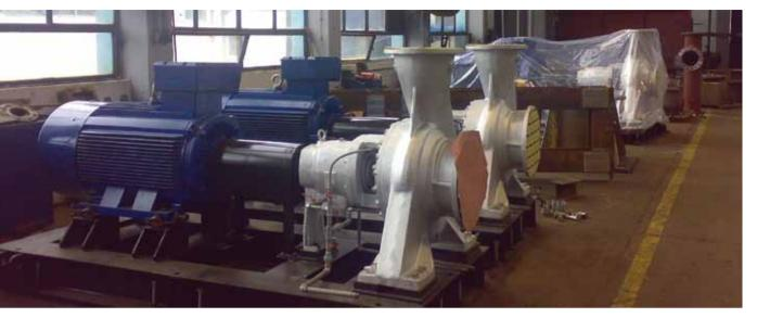
Manufacturing and delivery of 3 End Suction Centrifugal pumps for transport of cold and hot water for the needs of Belgrade Heating Plants, Serbia
