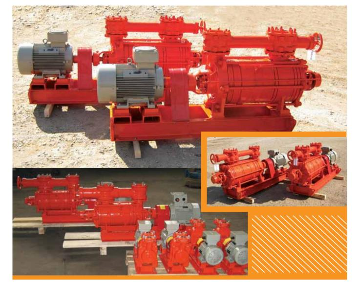
The main aim of this project was to produce and install self-priming multistage centrifugal petrol transfer pumps at NaftaChem, Novi Sad location Sremski Karlovci. The pumps are used for barge unloading.
