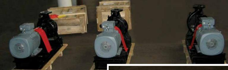
The main aim of this project was to produce and install self-priming multistage centrifugal petrol transfer pumps at EEE ANLAGENBAU GMBH, Germany. The pumps are used for transport of petrol products.
