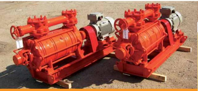
The main aim of this project was to produce and install self-priming multistage centrifugal petrol transfer pumps at plant station in Stip for oil and oil derivates. The pumps are used for decanting oil derivates.
