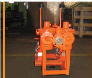
Production and delivery of 6 systems of Screw Spindle pumps with filter for unloading and transport of masut indented to be installed in Serbian heating plants
