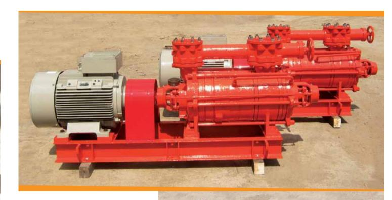
The main aim of this project was to produce and install self-priming multistage centrifugal petrol transfer pumps at Jedinstvo AD Sevojno, Terminal Smederevo. The pumps are used for transport of petrol products.
