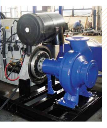
Production and delivery of Fire fighting diesel pump unit
