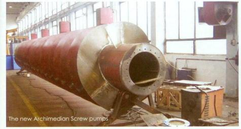
MZT Pumpi - Macedonia, one the leading manufacturers of industrial pumps for transport of water oil and derivatives in south-east Europe, has successfully produced 3 Archimedean screw pumps for the Environmental protection project for transport of untreated wastewater from east Skopje to a wastewater treatment plant.
