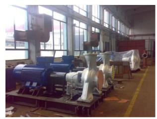
The pumps are designed for a bigger flow through them, the strongest pump having a capacity of 1700m<sup>3</sup>/h. All pumps can withstand water temperatures of up to 180 °C, which make them suitable for heating utility companies. The pumps are powered by electrical motors of different power, the strongest having a capacity of 710 kW.
